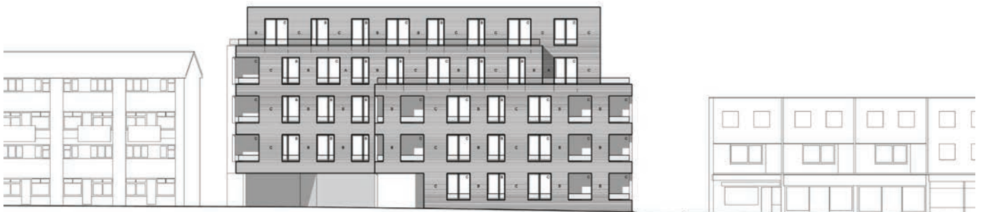
Elevation to show the relationship of the built facade and the adjoining three and four storey buildings
