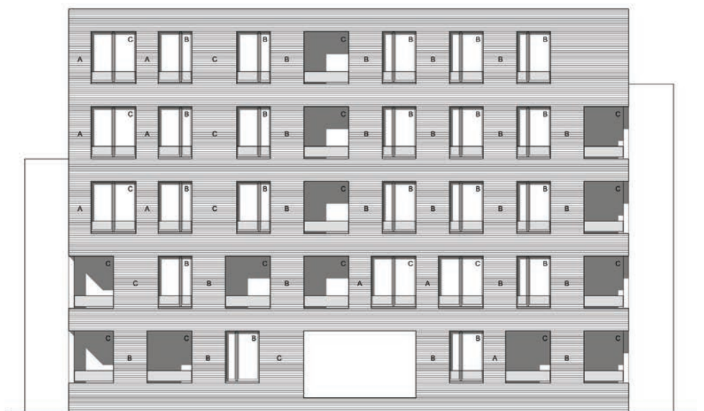
An early proportion study of the rear block courtyard elevation using the two chosen window proportions and the three pier sizes they relate to
